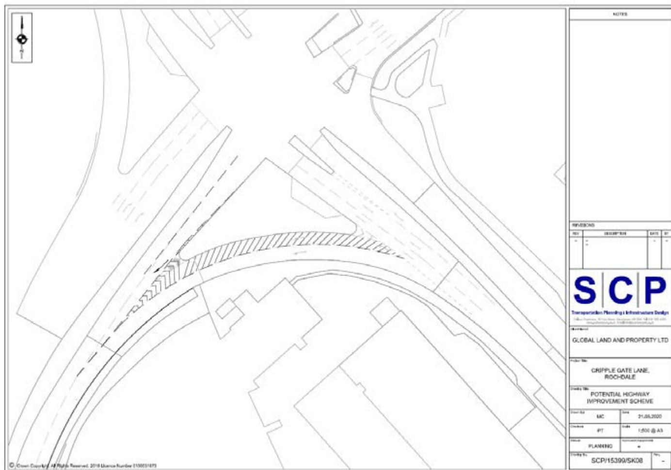
Figure 15. Proposed A664 (northbound) to A627(M) Free-Flow Movement - A664 Queensway / A664 Edinburgh Way / A627 (M) / Sandbrook Way Signal Junction [Illustrative/Typical Layout]
